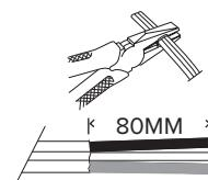
1. Measure and strip the cable 46mm for an inline connection or 80mm for an end of line connection. Conductor Range 1.0mm<sup>2</sup> to 2.5mm<sup>2</sup> solid/stranded to AS/NZS5000. DO NOT use for conductors outside this range.
