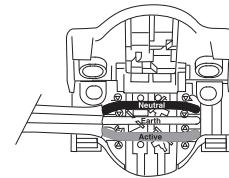
2. Put the cables into the slots according to the indicated colours as shown to ensure correct polarity.
